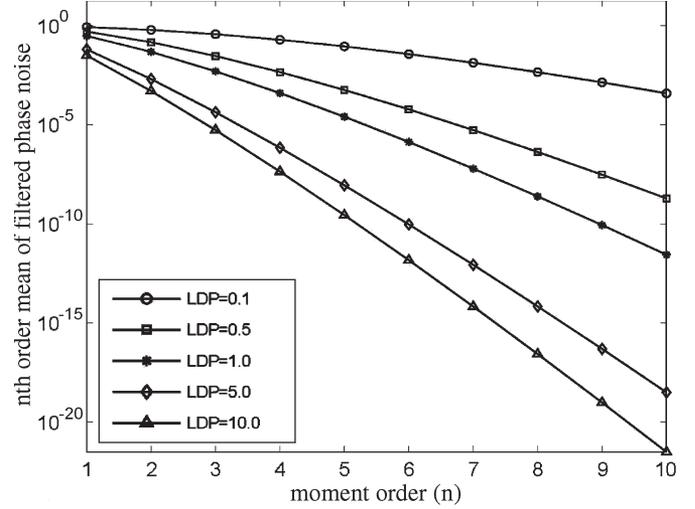
Fig. 3.  $n$ th-order mean of filtered phase noise for several values of the LDP.
