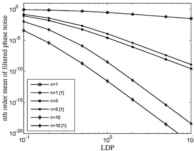
Fig. 6.  $n$ th-order mean of filtered phase noise as function of the LDP for several values of  $n$ . Comparison with the results of [1].
