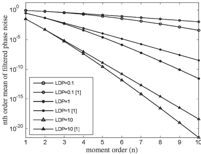
Fig. 5.  $n$ th-order mean of filtered phase noise for several values of the LDP. Comparison with the results of [1].
