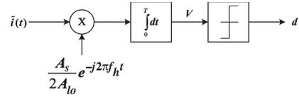
Fig. 2. OOK low-pass equivalent demodulator.
