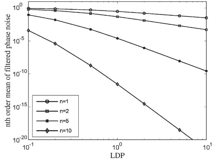
Fig. 4.  $n$ th-order mean of filtered phase noise as function of the LDP for several values of  $n$ .
